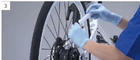
3 With the oil port still in the upper position, attach the syringe with its piston fully pushed in.
