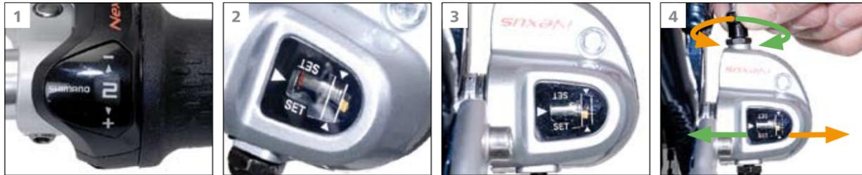
1 Shift up from gear 1 to gear 2.
