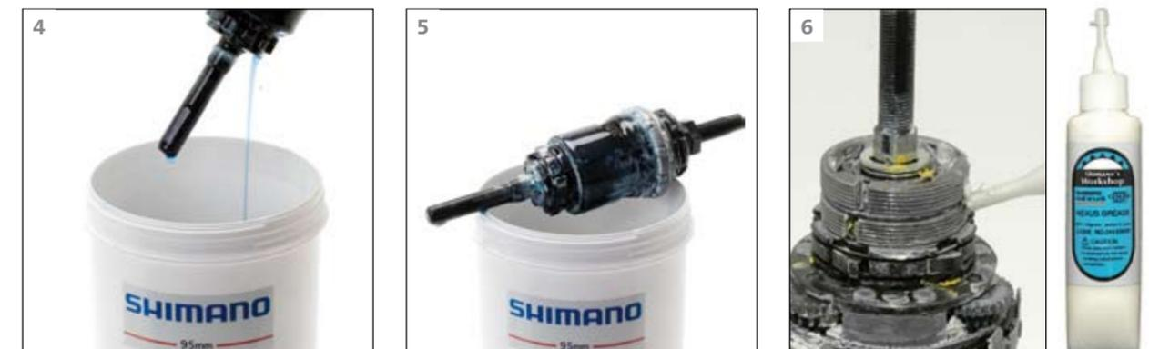
**4** Remove the internal unit from the oil.
