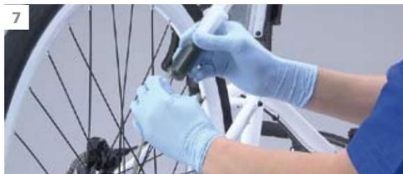
7 Carefully remove the syringe and tube containing the old oil.
