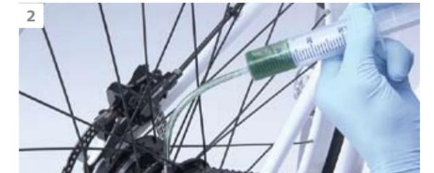
2 Assemble the bleed nipple with tube and attach the syringe. Push the piston slowly to inject the new oil into the hub.
