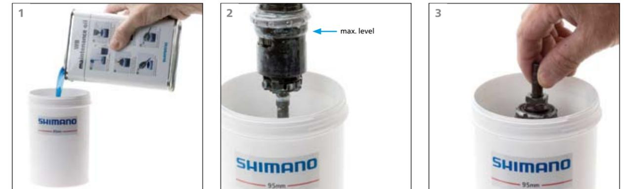
**1** Fill the dipping vessel with WB oil.
