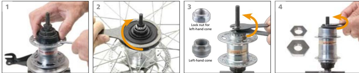
**1** Hold the two flat surfaces of the hub axle in a vice. **Note:** Do not damage the threads of the axle. Carefully remove the right-hand dust cap.
