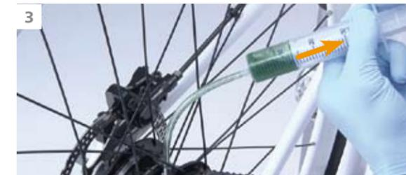
3 To reduce the pressure inside the hub, periodically pull the piston back a little.
