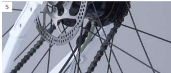
5 Wait 5 minutes until the oil has settled. Pull the syringe's piston slowly to drain all the old oil from the hub.
