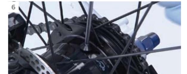
6 Reassemble the oil port bolt with O-ring and tighten it with a 3 mm Allen key. Tightening torque: 2-3 Nm.
