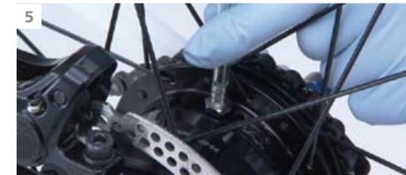
5 Remove the bleed nipple with O-ring and the tube.
