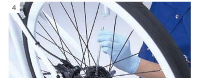
4 Once all the oil has been pushed out of the syringe, detach it from the tube to let the remaining oil in the tube flow into the hub.
