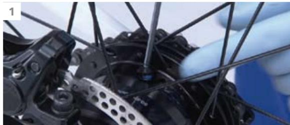
1 With the oil port in the upper position, remove the oil port bolt with O-ring using a 3 mm Allen key.
