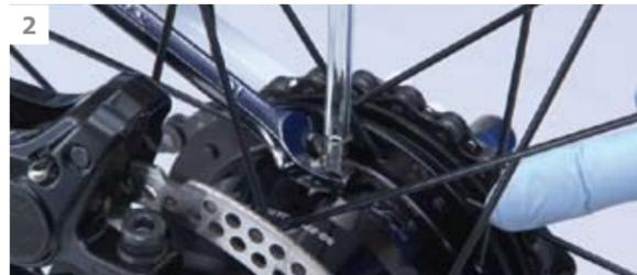
2 Attach the bleed nipple with O-ring and tube and tighten it using a 10 mm spanner. Tightening torque: 1-3 Nm.
